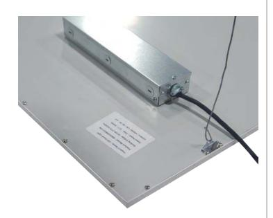
3) Reinstall cover plate on the driver housing and secure in place with two (2) screws. Secure the product to ceiling T-bars and attach to the ceiling with aircraft cable or wires capable of supporting 100 lbs. for hanging mount.
