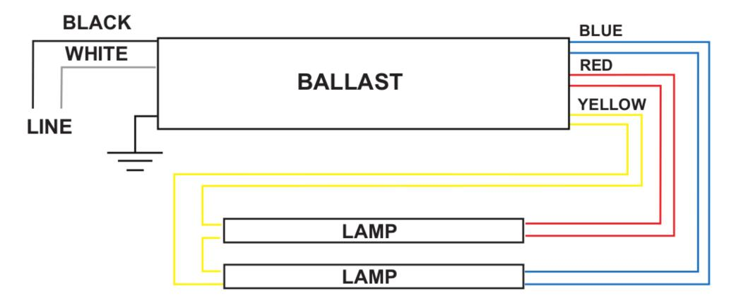
CAUTION: HIGH VOLTAGE: GROUND BALLAST CASE TO AVOID POSSIBLE SHOCK HAZARD. MOUNT LAMPS WITHIN 1/2 IN. OF GROUNDED METAL REFLECTOR.
