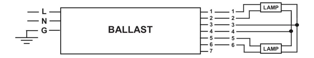
CAUTION: HIGH VOLTAGE: GROUND BALLAST CASE TO AVOID POSSIBLE SHOCK HAZARD. MOUNT LAMPS WITHIN 1/2 IN. OF GROUNDED METAL REFLECTOR.
