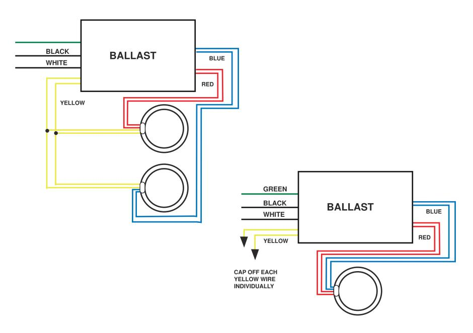
CAUTION: HIGH VOLTAGE: GROUND BALLAST CASE TO HELP AVOID POSSIBLE SHOCK HAZARD. MOUNT LAMPS WITHIN 1/2 IN. OF GROUNDED METAL REFLECTOR.
