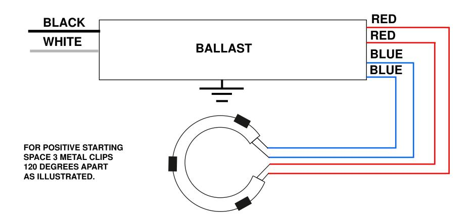
CAUTION: HIGH VOLTAGE: GROUND BALLAST CASE TO AVOID POSSIBLE SHOCK HAZARD. MOUNT LAMPS WITHIN 1/2 IN. OF GROUNDED METAL REFLECTOR.
