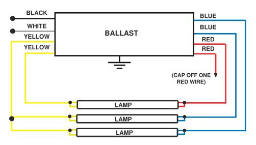
CAUTION: HIGH VOLTAGE: GROUND BALLAST CASE TO AVOID POSSIBLE SHOCK HAZARD. MOUNT LAMPS WITHIN 1/2 IN. OF GROUNDED METAL REFLECTOR.
